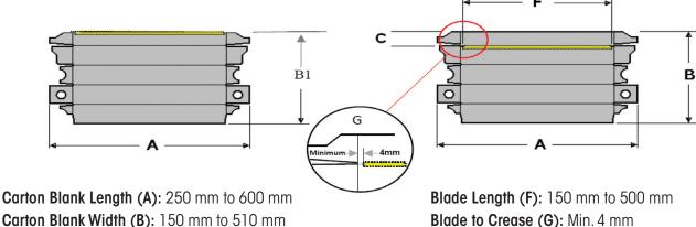
Carton Blank Width (B): 150 mm to 510 mm Carton Blank Width (B1): 150 mm to 440 mm
