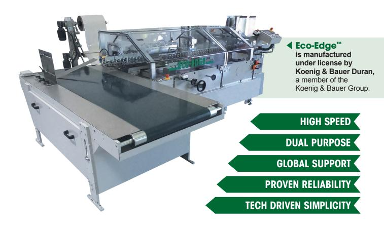
The **Eco-Edge™ 500s/500HM**, is a high-speed constant motion machine. Cartons are removed from the feed magazine by friction belts to the blade application station. The blade material is indexed at a right angle and taken from a reel that is advanced by servo operated drawing rollers, then cut to a pre-selected dimension by means of toothed upper and lower die arrangement.
